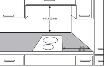
\*The clearance must meet or exceed the minimum recommended for both the rangehood and cooktop. Refer to the rangehood installation manual.
