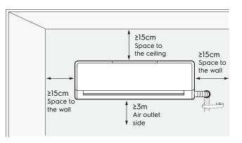
Please note! Dimensions to be used as a guide only. All customers MUST refer to the user manual supplied with the product for detailed installation instructions. © 2023 Electrolux S.E.A PTE. LTD. ELX\_DIM\_ESV183C3XB\_Oct23
