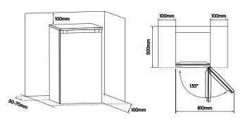
**Suggest:** It is advisable for there to be 50-70mm of space from the back to the wall, at least 100mm from its top, at least 100mm from its side to the wall and a clear space upfront to allow the doors to open 135°. As shown in follow diagrams.
