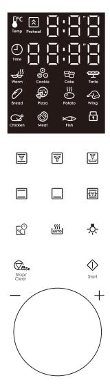
1. Start Press this button to START the oven. Stop/ Clear 2 Press this button once to STOP the oven. Press button twice to CLEAR oven current settings. Press button and hold for 3 seconds to activate/deactivate CHILD LOCK. Y 3.
