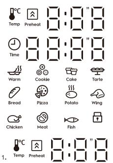
Temperature display, from 40°C-230°C, when In preheat phase, the "Preheat Indicator" wlll blinking.
