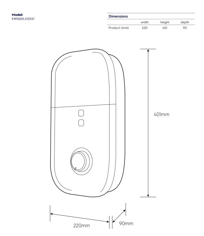
Please note! Dimensions to be used as a guide only. All customers MUST refer to the user manual supplied with the product for detailed installation instructions. © 2021 Electrolux S.E.A PTE. LTD. E\_DIM\_EWE601LX1DIX1\_Jun21
