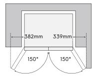
When positioned in a corner area, spacing of at least 382mm on the right hinge side and 339mm on the left hinge side will allow the doors to open enough to enable the removal of bins and shelves.
