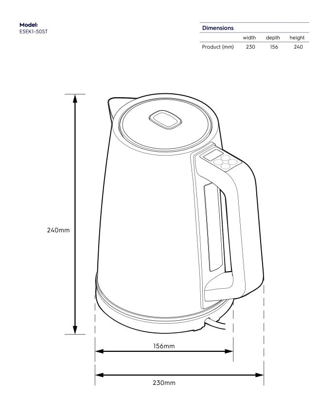
Please note! Dimensions to be used as a guide only. All customers MUST refer to the user manual supplied with the product for detailed installation instructions. © 2022 Electrolux S.E.A PTE. LTD. E\_DIM\_E5EK1-50ST\_Jun22
