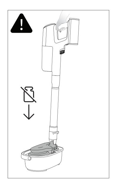
When washing the pads on your cleaning station, press the cleaner down only gently and keep it in an upright position. If you use too much force, the cleaner may switch off. This is a safety feature. If this happens, wait around 10 seconds, switch the cleaner on again and press it down with less force than before.
