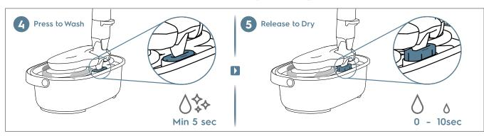
4 Gently press down the PRESS button to wash the pads. Hold the cleaner in an upright position. 下方向へ軽く押し洗浄 (5秒以上)
